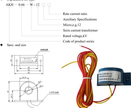
Note: Primary current flow from P1 to P2(Glue surface). The yellow second wiring is S2, the red is S1. The outlet length is 2m + 10cm.
