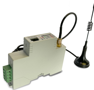
Figure 1 AWT100 Wireless communication terminal
