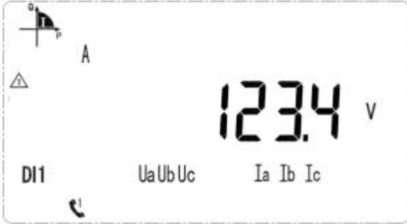
Voltage on A phase is 123.4V
